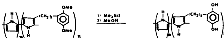
SCHEME 3 Conversion of Dimethoxyphenyl Group in the Copolymer to Dihydroxyphenyl Group
